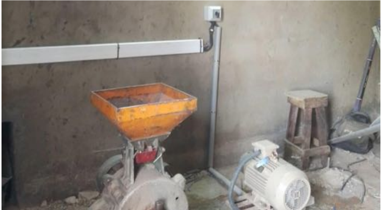
Figure 21 : First engine at the right-side powering peanut butter machine
