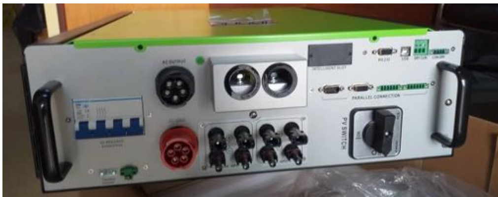
Figure 17 : Bottom view of the inverter
