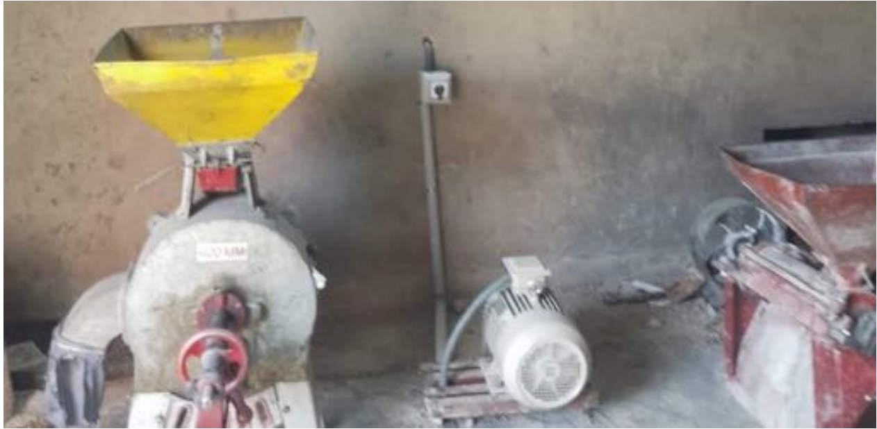
Figure 22 : The second engine in the middle powering either the dehusker of maize at its right or the maize milling machine at its left
