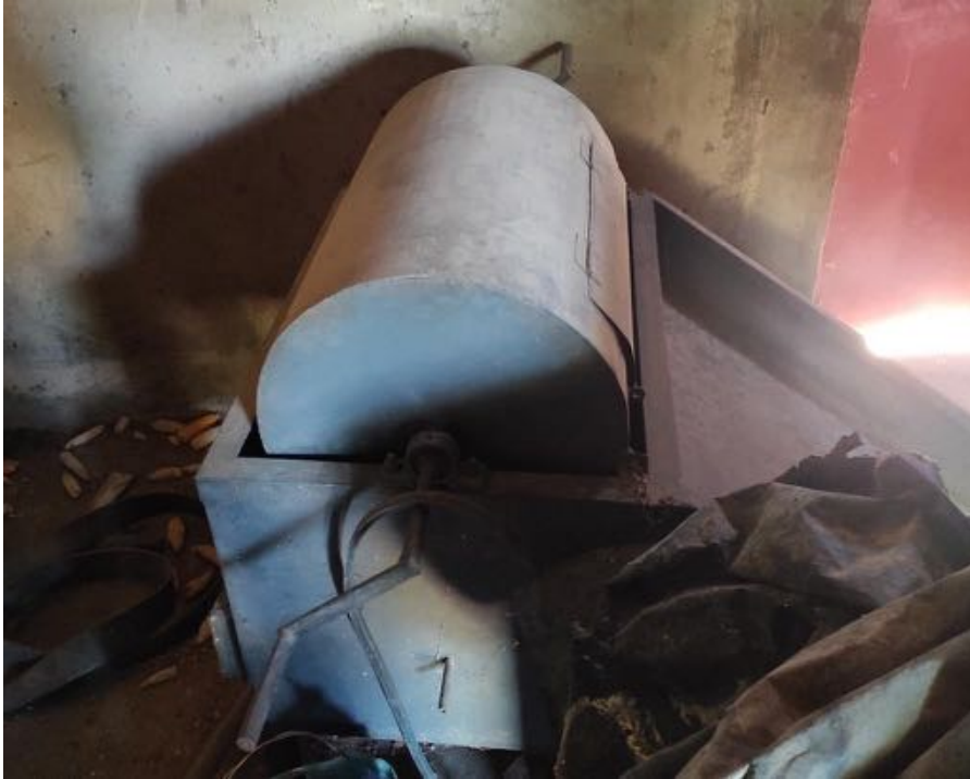
Figure 6 : A shea roaster (run with wood)
