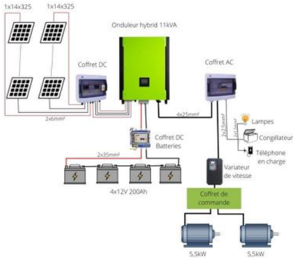
Figure 9 : Schematic of the system
