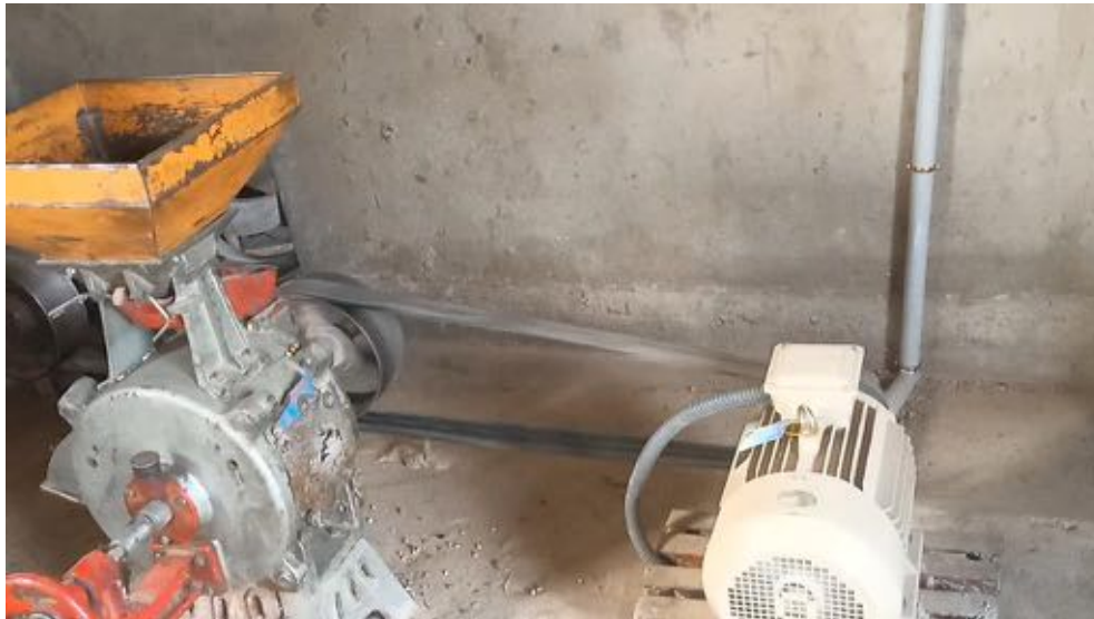
Figure 28 : Engine running the peanut butter machines
