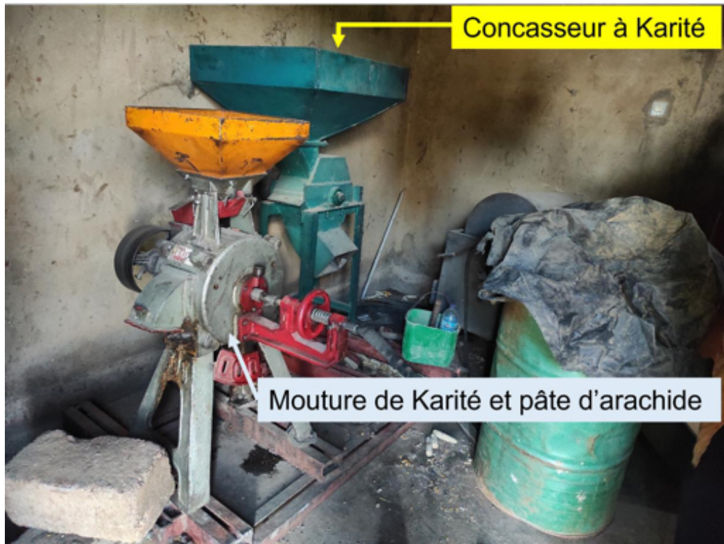
Figure 2 : A Crusher (mill with 300 mm stone wheels for oilseeds – shea and peanut) and a hammer crusher for shea.
