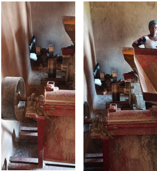
Figure 3 : An "Engelber" type huller to remove corn bran and a mill to produce corn flour.
